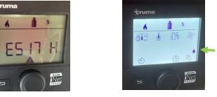
To use electricity ensure the caravan is plugged into an operational electrical connection. Check the 240 volt power source is functioning by plugging in the electric jug. Set the 3rd icon to ELEC2 and If the error code is not blinking turn on the heating hot water system.
