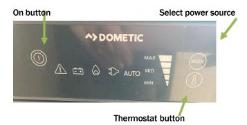
When using gas it can sometimes take a few minutes to light. If a warning triangle appears it is likely caused by an airlock please unscrew the gas regulator give it a tap and reattach it. This usually clears an airlock.
