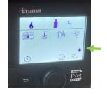
To use electricity ensure the caravan is plugged into an operational electrical connection. Check the 240 volt power source is functioning by plugging in the electric jug. Set the 3rd icon to ELEC2 and If the error code is not blinking turn on the heating hot water system.
