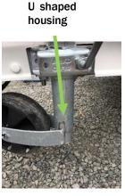
**Stabiliser Legs:** Use the winder tool to raise and lower the stabiliser legs. The stabiliser legs must be up while traveling and down when the caravan is disconnected from the car. The fitting nut for the two rear stabiliser legs is located at the rear of the caravan and the fitting nut for the stabiliser at the front of the caravan is on each side toward the front of the caravan. The rear legs must be down before entering a caravan disconnected from the car or the caravan will tip.
