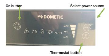
When using gas it can sometimes take a few minutes to light. If a warning triangle appears it is likely caused by an airlock please unscrew the gas regulator give it a tap and reattach it. This usually clears an airlock.
