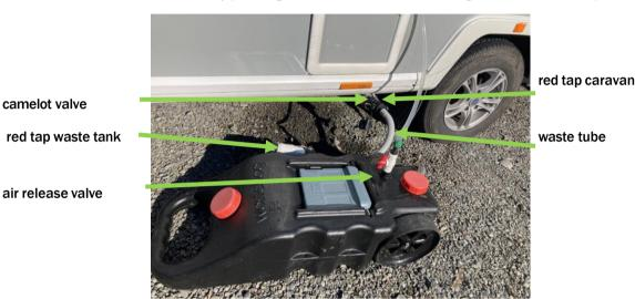
Ensure the red tap on the waste bin and the red tap on the caravan connection are open ie running in the same direction as the hose. There is a small breather pipe which acts as a air release valve on your waste bin. Ensure the cap on the end of this is removed to allow air to escape as the tank fills. The cap should be returned for travel if there are contents in the bin, to prevent leakage.
