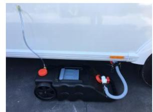
If it is not already connected connect the air release valve (clear plastic tube) by depressing the gold fitting or hose connection fitting as appropriate. If you wish you can connect the end of the air release pipe to the plastic hook on the caravan to keep it out of the way.
