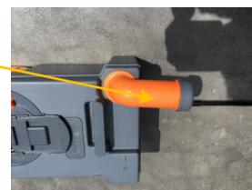
Slide this lid and rotate this button to place a hose inside the cavity to clean it. It must come back empty and clean.
