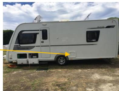
Empty your toilet cassette by removing it from the cavity, closing the top lid and emptying via pipe. Rinse out and replace.
