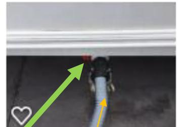
Connect the waste water pipe between waste water container and caravan. Ensure the tap under the caravan is in the open position. (see image)
