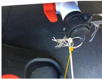
Remove the waste water plug from the fitting in the caravan. It must be fitted for travelling
