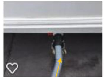
Connect the waste water pipe between waste water container and caravan
