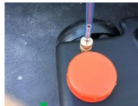
Connect air escape valve (plastic tube) by depressing on the gold fitting. Connect the end of the valve to the plastic hook on the caravan by the loop at the end of the plastic level indicator pipe.
